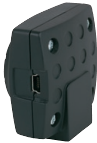
The USB port is provided on the side to save space
